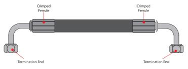
Fig. 3 - Complete hydraulic hose assembly
