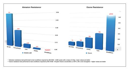
Fig. 5 - Abrasion and ozone resistance performance of Manuli cover compounds
