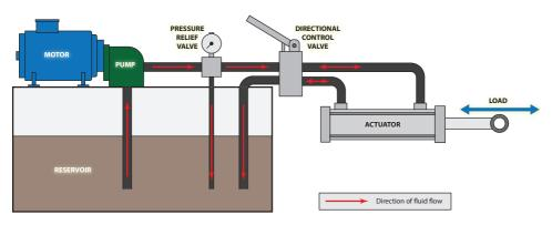
Fig. 1 - A simple hydraulic circuit
