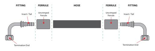
Fig. 2 - Individual components of a hydraulic hose assembly
